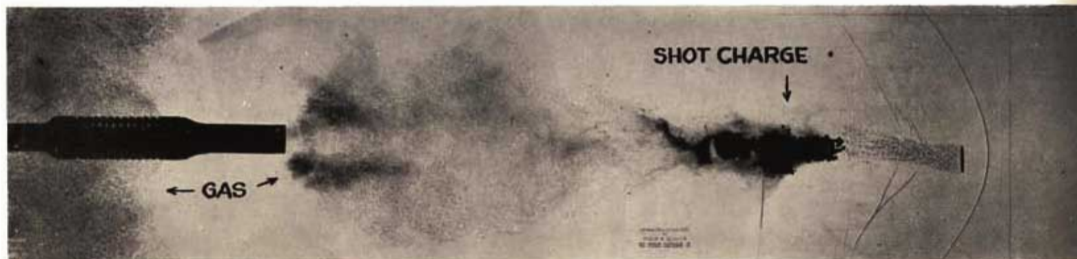
Shot charge passing through Cutts Comp is shown in spark photos made during design period. In first photo, top wad has sealed choke tube and expelled air from muzzle, while in second view shot charge has been shaped by tube and is just emerging. In bottom view over-powder wads fall behind shot, avoid "blown patterns" and missed birds.
