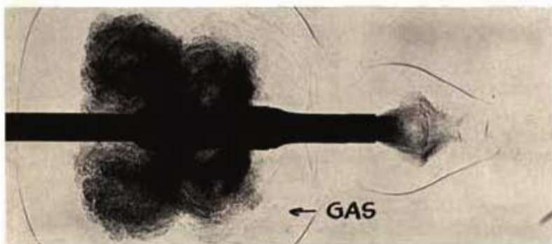
Shot charge passing through Cutts Comp is shown in spark photos made during design period. In first photo, top wad has sealed choke tube and expelled air from muzzle, while in second view shot charge has been shaped by tube and is just emerging. In bottom view over-powder wads fall behind shot, avoid "blown patterns" and missed birds.
