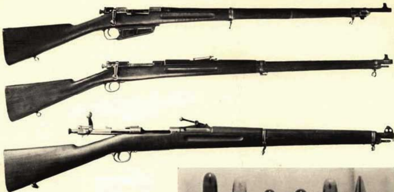
Early Springfields made during development of cartridge were M1900 with Mannlicher magazine, Lee-type cut-off; M1901 with rod bayonet, Mauser magazine; original M1903.
